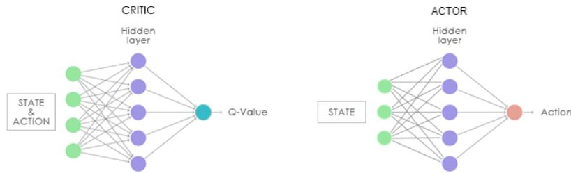
FIGURE 3.3: The Actor-Critic architecture. Two networks are used, the actor (or policy) network for selecting actions, and the critic (or value) network for training the policy.
